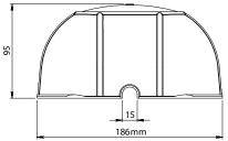
**TH 095** has been specifically designed for use in sloped ceilings or fitting into a 100mm floor. The overall height of 95mm allows for fitting where height is restricted and maximum space for insulation is required.
