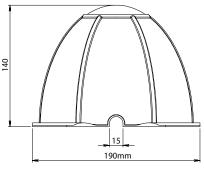
**TH 001** is the most popular product in the Thermahood range as it can be easily fitted over most downlights. Squared sides allows for fitting close to joist and there are four corner flanges for fixing in position.
