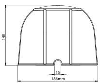
**TH 140** has more space inside due to the square shape and has no flange, this allows for fitting close to joist or rafters. TH 140 can be used with larger downlights and with downlights which have the connector block fixed at 90 degrees to the light fitting.
